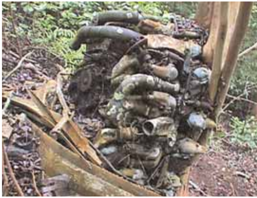
Above, the U.S. white star insignia can be seen on the left wing fragment. Left, one Wright R3350-30W engine rests next to a tree. Below, the BuNo is visible on the tail section. Below middle, part of the word NAVY remains on the left wing. Below bottom, the 20mm tail gun turret.
